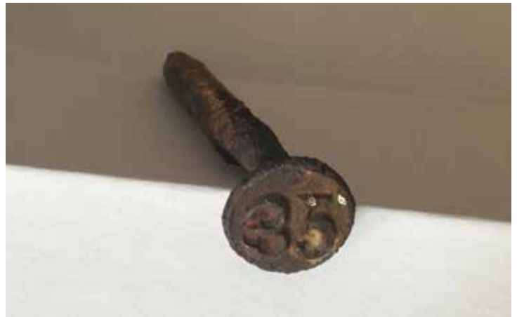
85 year old PG&E nail with "35" engraved on its head
