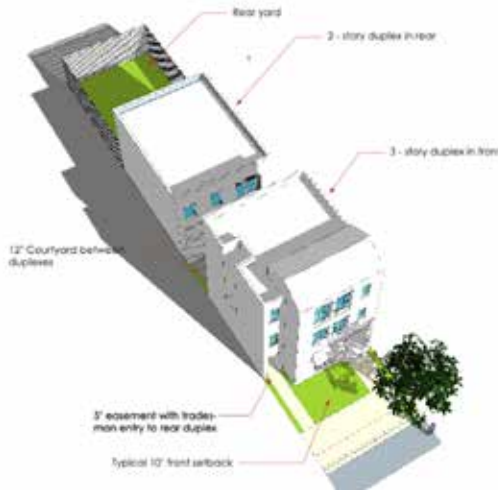
What Could a Split Lot Look Like to Add a Duplex Under SB 9 in Miraloma Park? Option 1 – Demo the existing house and construct duplex at the front and rear (60/40 lot split) for 4 units.
